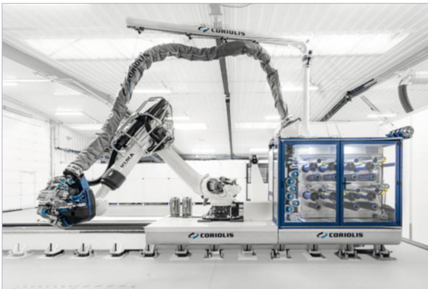
Fig. 1: The C1.2 is a compact, easy-to-use and versatile machine for depositing multi-materials (thermoset, thermoplastic and dry fibre)
