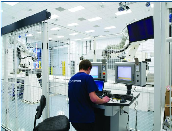
A technician with Coriolis Composites controls the automated fiber placement machine at the National Composites Centre in Bristol, England.
