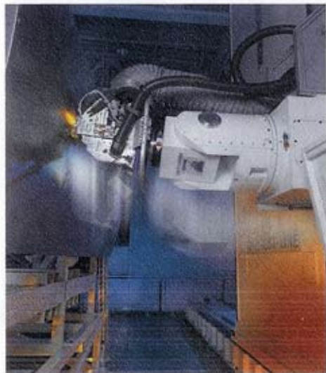
Innovation: new fibre placement machine to be used for manufacturing complex composite parts.
